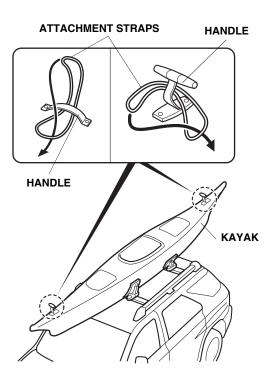
12. Attach one ratchet hook to the front attachment strap, and one ratchet hook to the rear attachment strap. Attach the front hook to the front bumper beam or tow hook. Attach the rear hook to the rear bumper beam or the trailer hitch. Secure the kayak to the vehicle by pulling the rope through the ratchet hooks.
