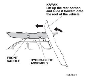
4. Adjust the distance of the saddles and hydro-glide assemblies to the same width as the kayak, then secure the saddles and the hydro-glide assemblies by tightening the knobs you installed in steps 1 and 2.
