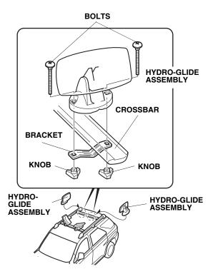
3. Rest the front of the kayak on the hydro-glide assemblies. Standing beside or alongside the kayak, lift up the rear portion if the kayak and push it forward, sliding on the hydro-glide assemblies and saddles. Make sure the kayak reaches the front saddles before you lower it.
