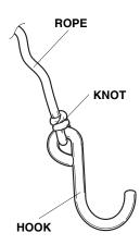
Route the other end of the rope through the bottom of the ratchet hook in the direction shown, and turn the spool until the rope end comes out of the ratchet.
